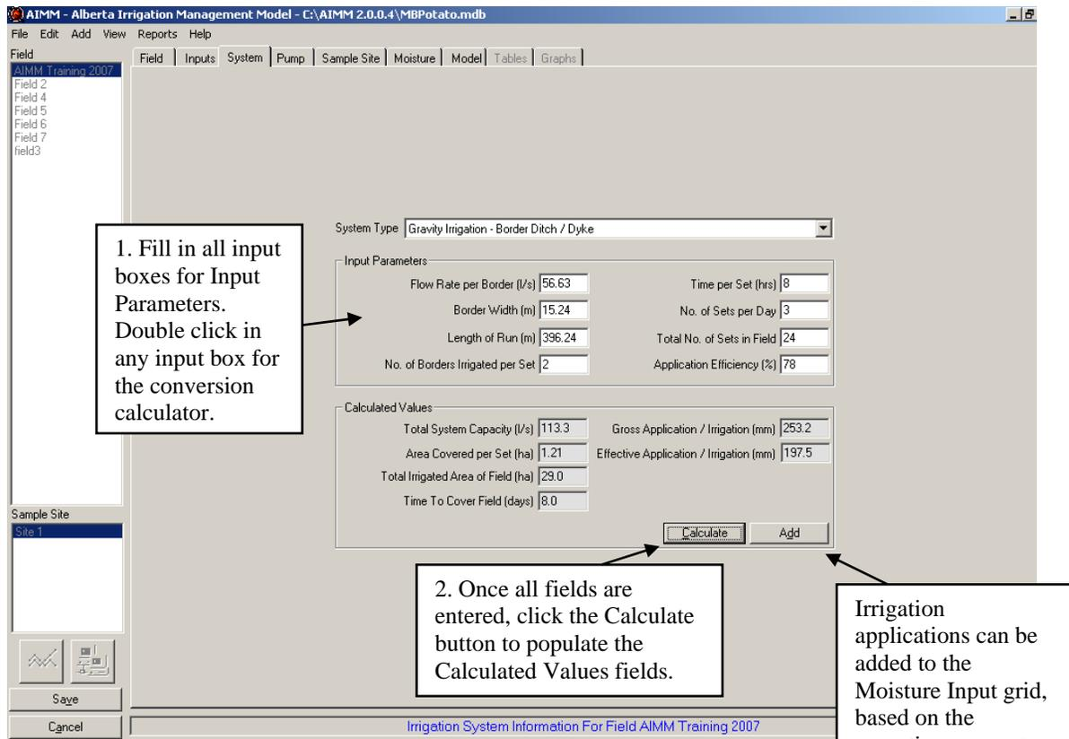
Figure 29. Data requirements for border dyke irrigation under "System" tab.
